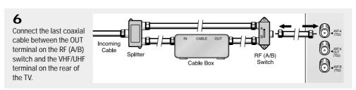
After you've made this connection, set the A/B switch to the "A" position for normal viewing. Set the A/B switch to the "B" position to view scrambled channels. (When you set the A/B switch to "B," you will need to tune your TV to the cable box's output channel, which is usually channel 3 or 4.)
